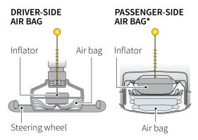
2 Inside the **inflator**, a rapid chemical reaction produces gas that fills the air bag within milliseconds.
