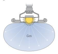
3 Shortly after, the gas quickly dissipates through tiny holes in the bag, deflating it so the driver can move.
